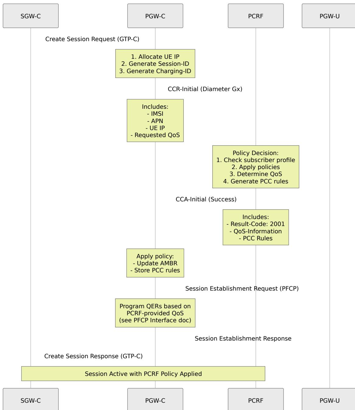
**Note:** QoS parameters from PCRF are translated into QERs (QoS Enforcement Rules) and programmed into PGW-U via PFCP. See [PFCP Interface](#) for QER details.
